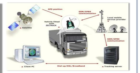
IVMS is a system providing management functions which allows companies to remove or minimize the risks associated with vehicles and goods owned by the companies.
